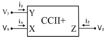
Fig1: Basic CCII+ current conveyor voltages and currents. It is a three port device with the following equations:
