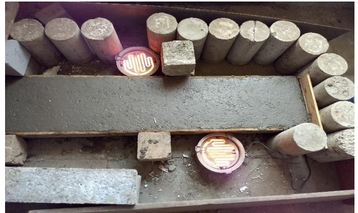
Fig 4 curing of slab
