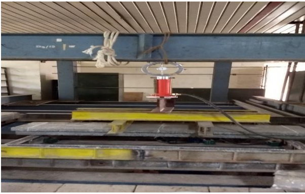
Fig 5 test setup for double T slab
