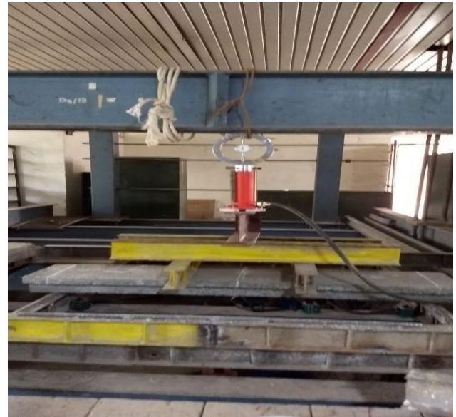
Fig 5 test setup for double T slab
